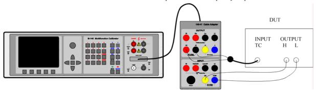
Function setup: Calibrator T TC function
