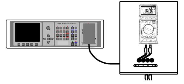
Optional current coil can extend the calibrator's current range to 1000 A. The coil can be used for calibration of both DC and AC ammeters. The clamps of the ammeter must be positioned in angle 90° to the coil. When using the current coil, no steel or other magnetic objects must be present in the vicinity (50 cm) of the current coil, as they would deform the magnetic field and cause big calibration error.
