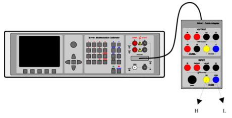
The multimeter allows the measurement of small DC voltages in the range of 0 to 2 V. 140-41 cable adapter is required. The signal to be measured connects to Hu/+mV and Lu/-mV terminals. Lu/-mV is the common terminal of the multimeter. To activate the measurement, select mVDC function mode using METER button in the function menu and press INPUT to measure the input value.
