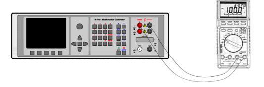
Truncated waveform with defined distortion can be used for testing of multimeters
