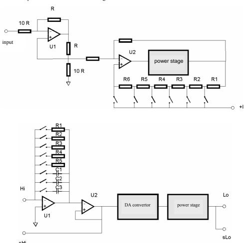
Hi and Lo are calibrator's output terminals. The stage including U1 operating amplifier converts voltage to current. U2 is a separation amplifier. R1 to R5 and C1 to C3 are range impedances. DA converter has 0 to +1 and 0 to -1 conversion ration and allows the simulation of resistance and capacitance values different from the range impedances. The output stage increases the permitted current load of the output.
