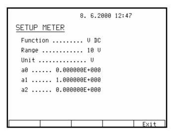
When the multimeter is being set-up, measurement cannot be initiated. Measurement can only be initiated after the menu is left using the INPUT button.
