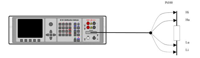
Connection of Pt - 100 by using the 140-41 cable adapter
