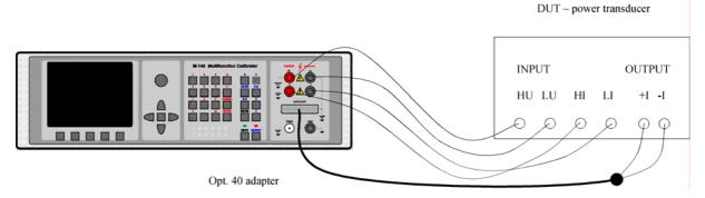
Function setup: Calibrator P function (voltage, current, power factor, frequency)
