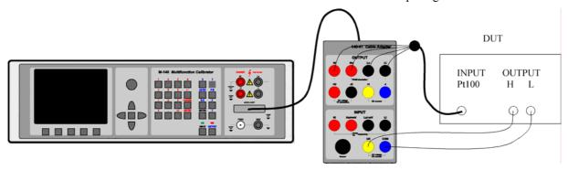
Function setup: Calibrator T RTD function
